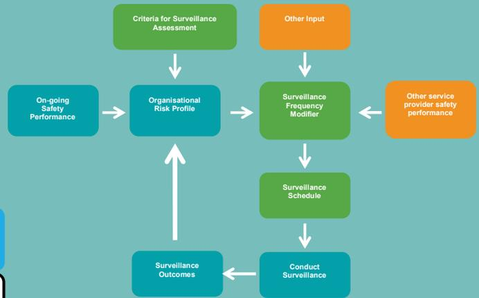
Fig. 3 - Safety Data and Risk-based Surveillance Concept
