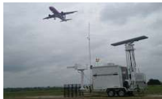
Figure 5 - A bird detection radar
