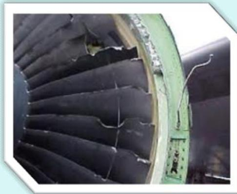
In December 2013, there were 3 confirmed bird strikes for Nadi – one of which cause \$36,000 worth of damage to fan blades on a Fiji Airways aircraft.
