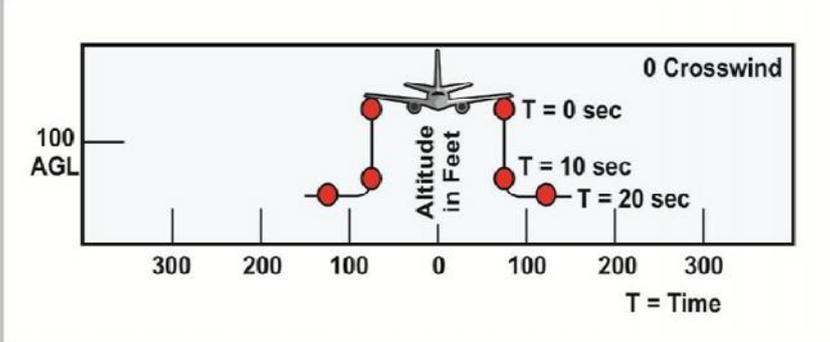
d. **Lateral Movement.** When the vortices of large aircraft sink close to the ground (within 100 to 200 feet), they tend to move laterally over the ground at a speed of 2 or 3 knots at an altitude of slightly less than one-half the wingspan (see Figure 6, Movement of Vortices from Low-Flying Large Aircraft).
