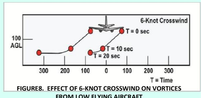
FIGURE8. EFFECT OF 6-KNOT CROSSWIND ON VORTICES FROM LOW FLYING AIRCRAFT
