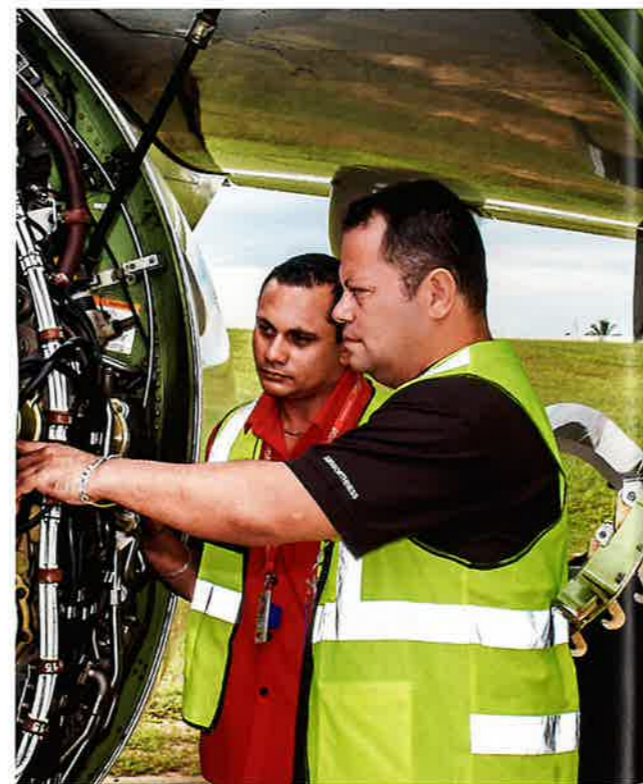
CAAF Airworthiness Inspector Anare Ravulo and Fiji Airways Engineer Israfil inspecting the pneumatic system on the B737-800.
